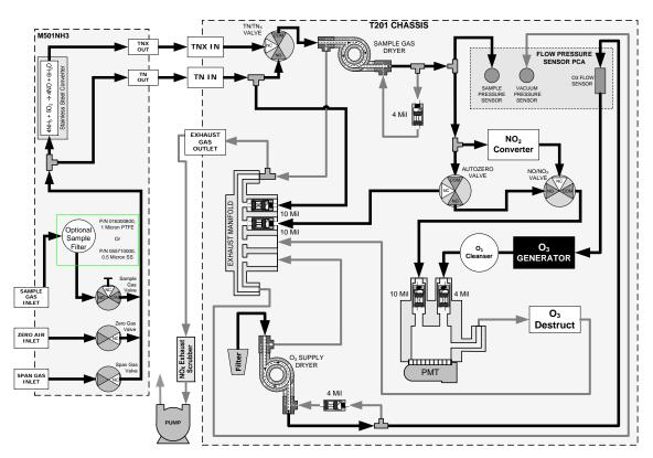
Figure 1-3. T201 and M501 NH<sub>3</sub> with Zero and Span Valve Options Pneumatic Flow
